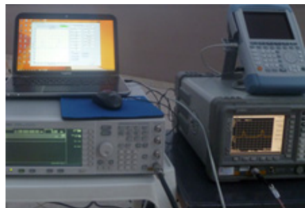
Fig. 5. Capturing of a real UMTS signal from Agilent E4407B Spectrum Analyzer
