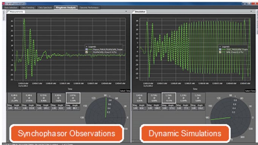
Fig. 8.11 Dynamic model validation using synchrophasor measurements (left), along with simulated reconstructions (right)
