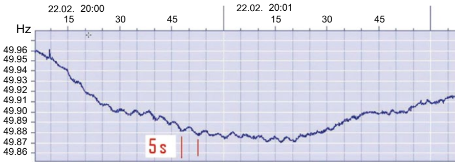
Fig. 4.1 Example for frequency measurement with PMU
