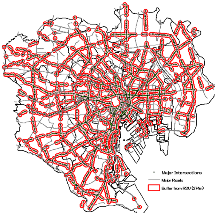
Fig. 4. WAVE RSU setting in Tokyo 23 wards [14]
