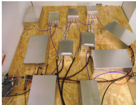
Fig. 2. Physical topology of Ko-TAG emulator
