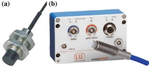
Fig. 5.26 Two commercially available eddy-current sensors. Photos courtesy of Lion Precision, USA and Micro-Epsilon, Germany
