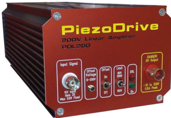
Fig. 8.16 Piezodrive PDL200 voltage amplifier used to drive the actuator
