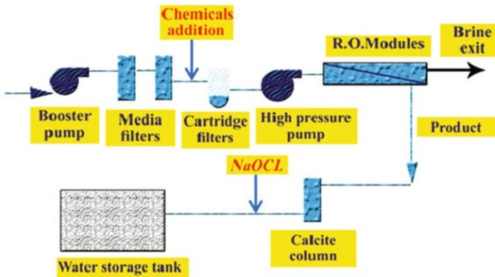
Fig. 7 Basic components of RO plant (Source: Authors)
