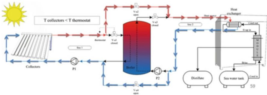
**Fig. 12** Schematic representation of the operating configuration 1 (cold hours of a sunny day): Solar energy is directly used to power the MD plant [31]
