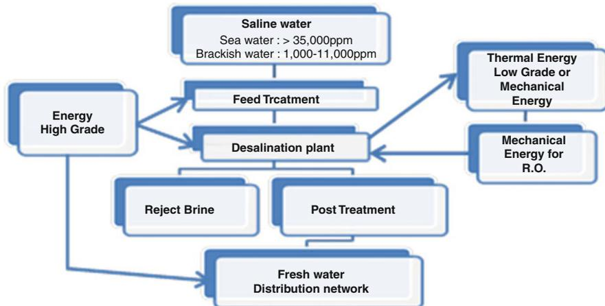
Fig. 1 Water and energy flow diagram of a desalination unit (Source: Authors)
