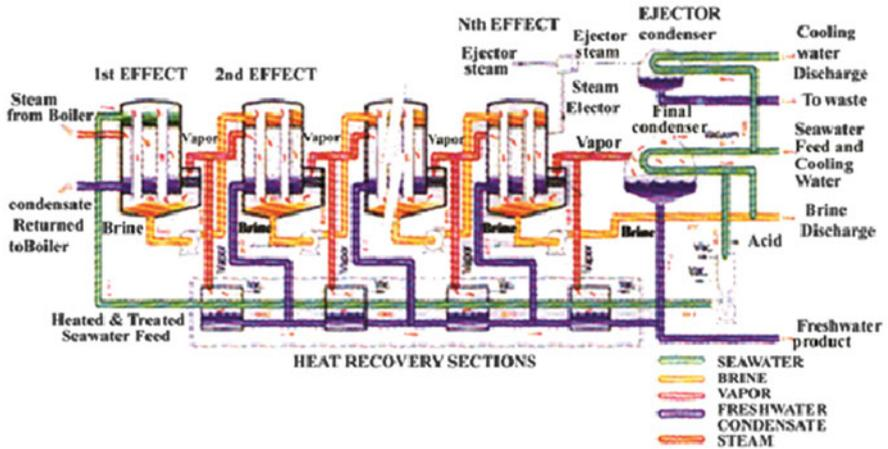
Fig. 4 Typical flow diagram of Multi-Effect distillation plant—Horizontal falling film plant [18]
