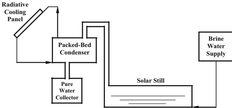
**Fig. 10** Schematics of the solar still and condenser [27]
