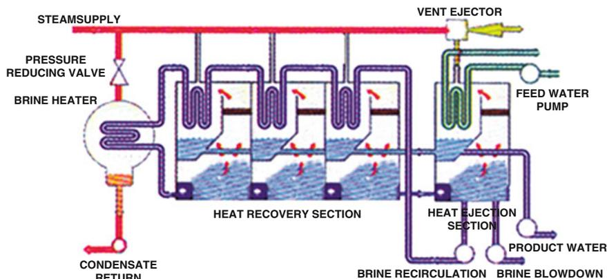
Fig. 3 Typical flow diagram of Multi-Stage Flash distillation plant [17]
