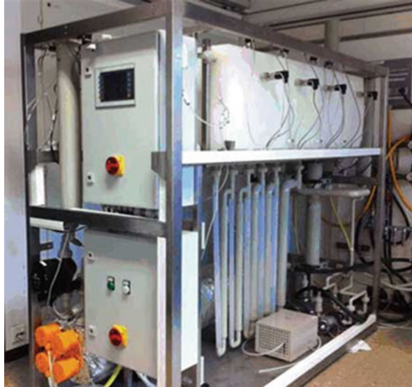
Fig. 16 The IBM HCPVT system's heated waste water is diverted to a desalination system, where it vaporizes and purifies saltwater (Courtesy of International Business Machines (IBM) Corporation, ©International Business Machines Corporation [44])
