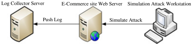
Fig. 1. Architectural Diagram for Simulation Attack and Web Log Collection
