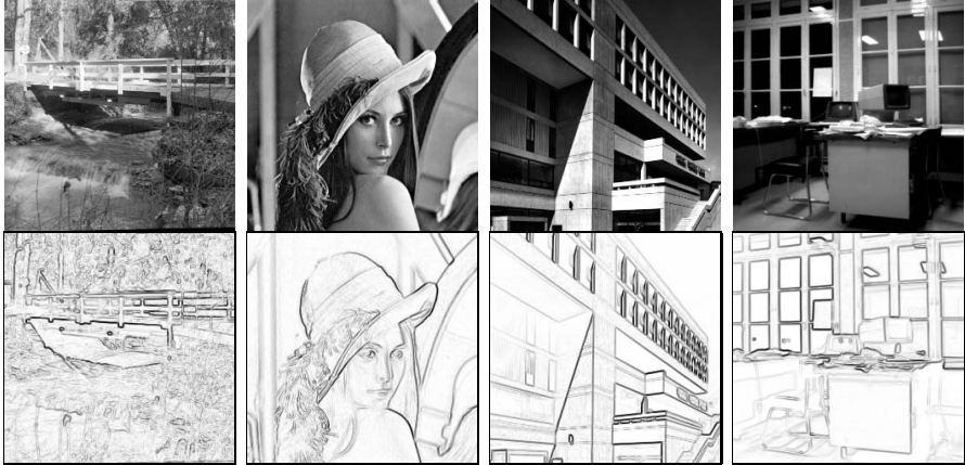
Fig. 5.3 Sample test images containing indoor, outdoor, man-made and natural scenes. Also are shown the Sobel edge maps for comparison.
