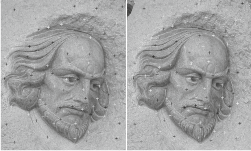
Fig. 4 The face image set , showing a facial stone carving captured from different distances and views of the scene. Corresponding control points in the image are also shown. The control points marked with a black '+' are used to determine the transformation function and the control points marked with a white '+' are used to determine the registration accuracy
