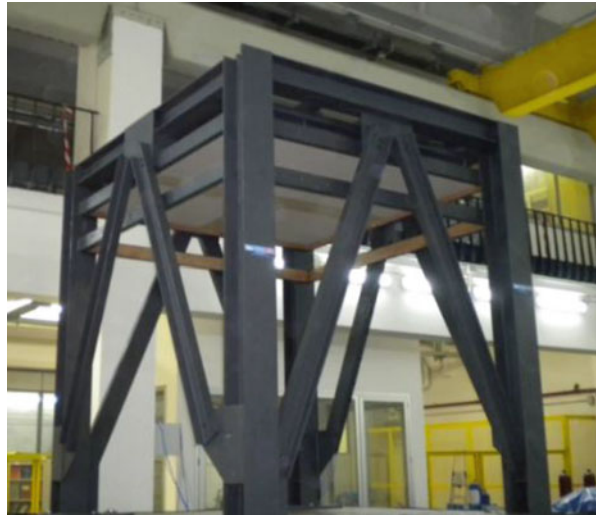
Fig. 7.2 Test frame installed on the shake table
