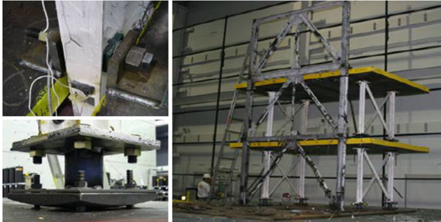
Fig. 5.1 Test setup – top left : mass to specimen connection; bottom left : hinge at the gravity frame; right : specimen
