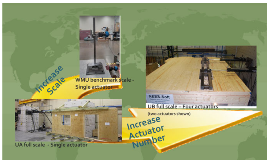
Fig. 9.5 Road map of hybrid simulation method development in the NEES-Soft project
