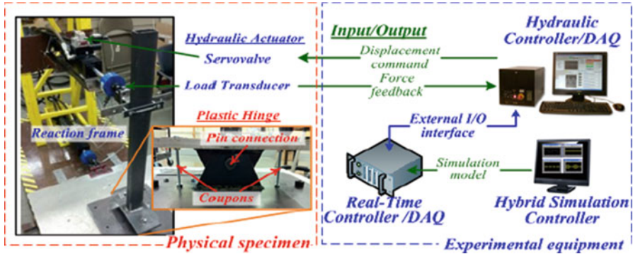
Fig. 9.6 Small scale WMU specimen and the LESS hybrid testing system
