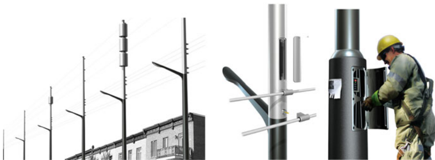
Fig. 4 Utility pole concept, housing components, with smart-detach system calibrated for weight overload during extreme weather conditions (student project 2008)
