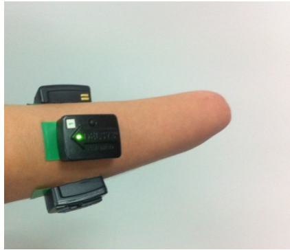
Fig. 5. Four bipolar sEMG electrodes were placed on the residual forearm of the transradial amputee in Strategy 2
