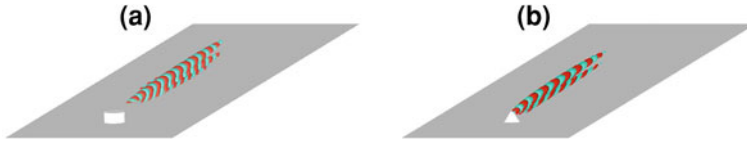
Fig. 3 Streamwise velocity component of the most unstable mode obtained at Re = 1,000 for the cylindrical roughness element (a) and the smooth one (b)
