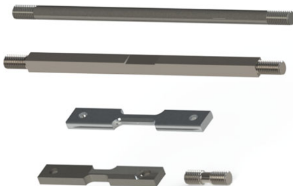
Fig. 3 Basic Sample designs used in XTMS experiments. Sample length range from 120 to 25 mm, and width from 14 to 5 mm
