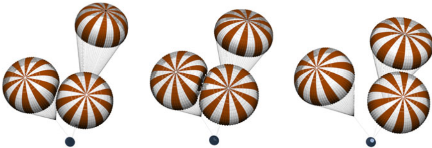
Fig. 11 A cluster of three parachutes at three instants during the FSI computation, with contact between two of the parachutes
