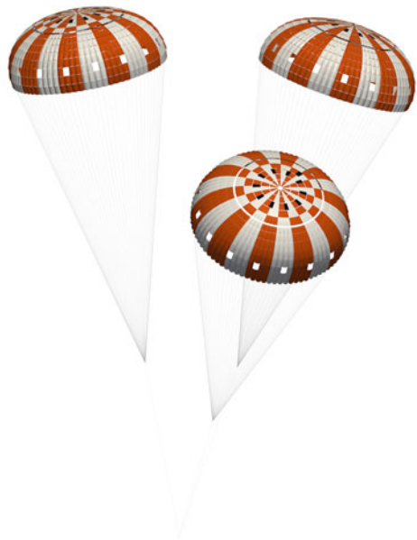
Fig. 12 Parachute disreefing from [55]: side and bottom views
