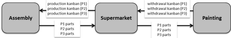
Fig. 4. Kanban-based pull system as interactions involving a supermarket as an intermediary subject
