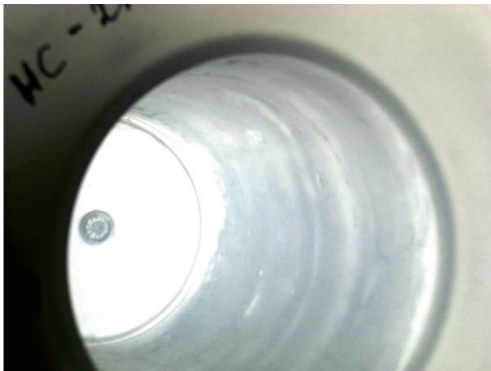
Fig. 14.9 Surface crack formation after 36 months IP/DP box exposure (view inside the PP hat from bottom to top)
