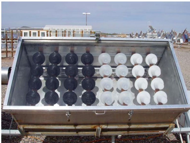
Fig. 14.1 All four basic materials (stabilised with 0.22 % N 30) had been exposed in an IP/DP box in Phoenix, for varied durations (3–36 months)
