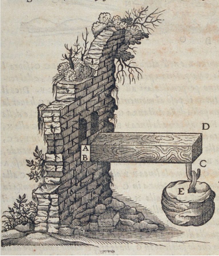
Fig. 12 Cantilever beam (From Galilei 1638, 114)
