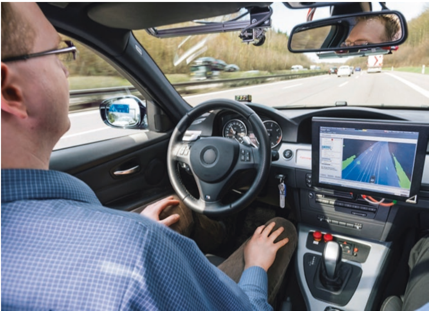
Fig. 7 A Bosch engineer supervising an automated vehicle test drive. The safety concept worked up for the test campaign was tested and approved by TÜV Süd. [2]
