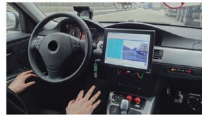
Fig. 3 Integrated cruise assist combining longitudinal and lateral assistance for partially automated driving
