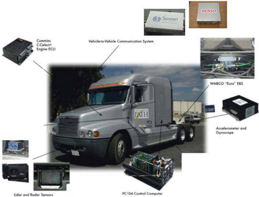
Fig. 2 Sensors and actuators installed on three trucks
