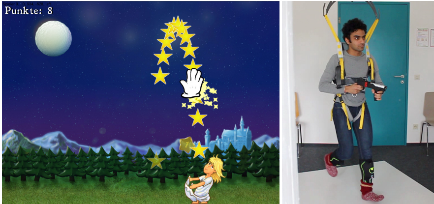
Fig. 1. Exergames examples. Left: screen shot of star-money, a game for PD patients, right: device for suspended walking interface for the SPortal game.
