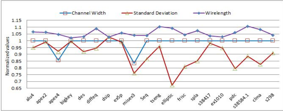
Fig. 1. Comparative results of Channel width, Standard deviation and Wirelength for diffusion based placement algorithm normalized to the respective results from VPR’s placement algorithm for cluster size N=1
