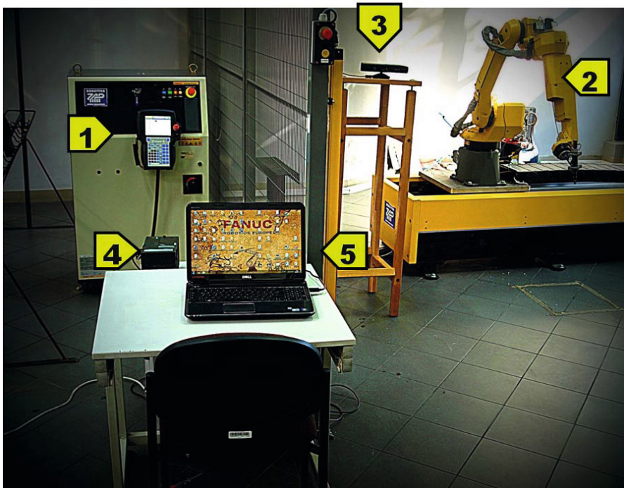
Fig. 3. Laboratory stand for human gestures robot control. 1 - Robot controller, 2 - Industrial robot, 3 - Kinect motion sensor, 4 - PLC, 5 - PC unit
