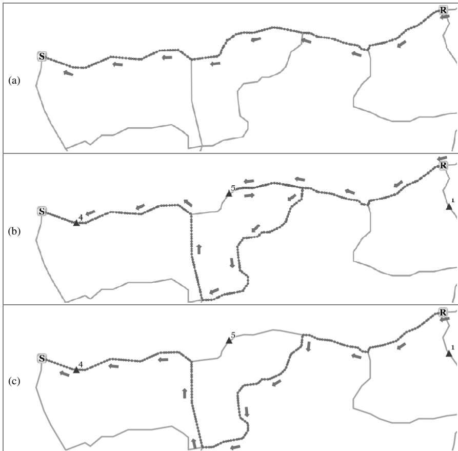
Fig. 3. Paths for vehicle 4 to traveling (a) the benchmark scenario (no travel barriers), (b) scenario 2, and (c) scenario 3 (the triangles are travel barriers, the arrows point the vehicle's movement direction, and the dots are the positions of the vehicle at each click simulation time)
