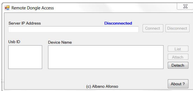
Fig. 3. Generic graphical user interface (GUI) developed for USB/IP client
