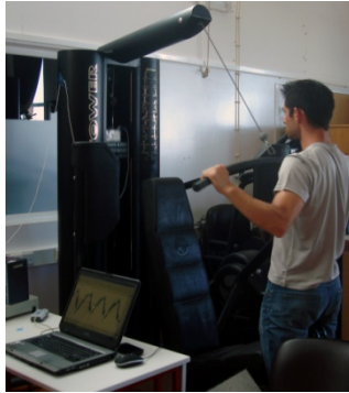
Fig. 1. Motion capture using accelerometers LIS302DL and TSD109F, coupled in a latissimus machine
