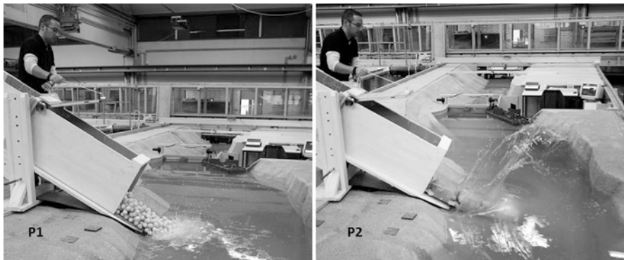
Fig. 8.8 Physical set-up golf balls (left) and skateboard (right)
