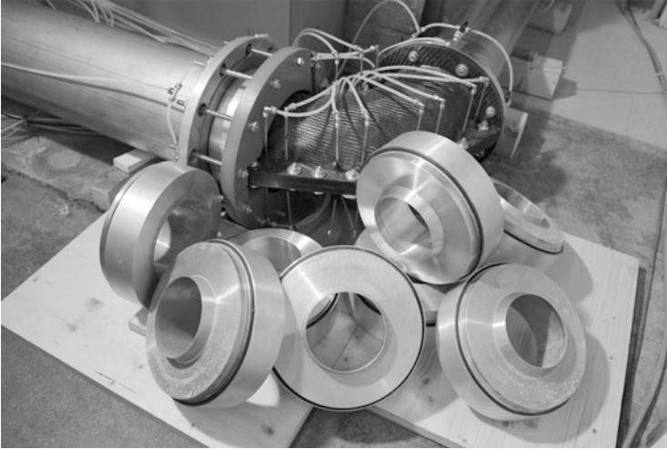
Fig. 8.3 Scale model test including the additional orifices
