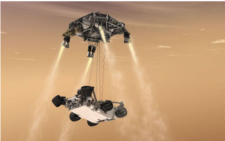
Fig. 45.3 The Curiosity Mars rover was landed by a rocket-powered hovering sky crane. Getting all this hardware to this situation is a system problem, not merely a project. Image credit: http://mars.jpl.nasa.gov/m2020/images/PIA14839-fi.jpg
