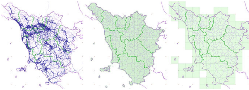
Fig. 7 (Left) A sample of the trajectory dataset used for the experiments. (Center) A partition based on a regular grid with cells of size 2,000 m. (Right) A partition with a grid with 20,000 m cell size
