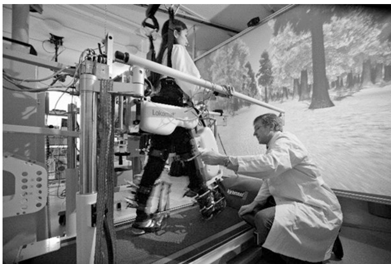
Fig. 10.1 The experimental setup described in this chapter, showing the Lokomat and video screens used for the interactive serious game
