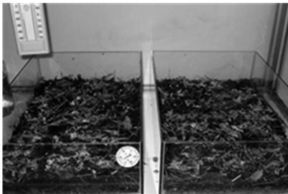
Fig. 4.3 Biobed system at laboratory scale used to evaluate pesticide degradation
