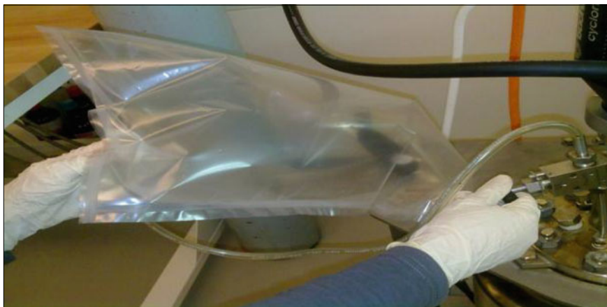
Fig. 47.4 Gas Fraction collected using tedlar bag
