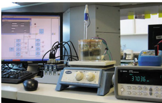
Fig. 52.3 Photograph of the brine water battery setup
