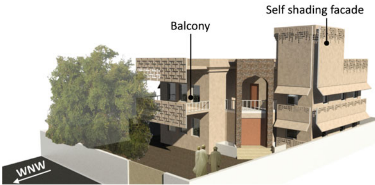
Fig. 20.14 Low EUI house after application of recommended shading (21 Oct at 14:00)
