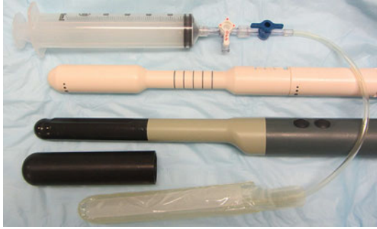
Fig. 1. Components used in the experimental setup. From top to bottom shown are (1) a syringe connected with the endocavity balloon (Civco); (2) rigid transrectal MRI coil (Hologic); (3) transrectal ultrasound probe (BK Medical); (4) custom fabricated TPX sleeve.
