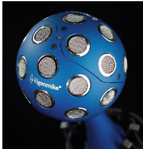
Fig. 11.6 “Eigenmike” with adjustable directional characteristics (Meyer and Elko [20])
