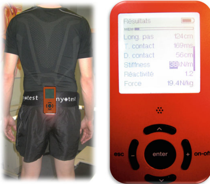
Fig. 8.12 Left: the Myotest™ accelerometer device is carried at the lower end of the trunk during running. Right: running mechanics and spring-mass variables (e.g. vertical stiffness) are displayed after a “run check” test
