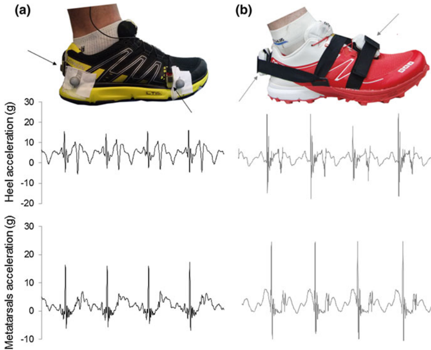
Fig. 9.1 Heel and metatarsals accelerometers' placements. Panel a accelerometers (ADXL150, Analog Device, USA) and placement used for the validation of the simple method (Giandolini et al. 2014). Panel b accelerometers (Agile Fox, Hikob, France) and placement used for field applications (Giandolini et al. 2015). For each placement, typical raw acceleration signals were presented
