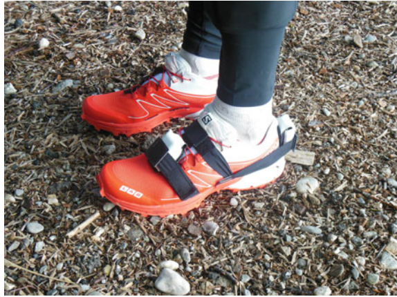
Fig. 9.4 Heel and metatarsals accelerometers' placements for a field experiment
