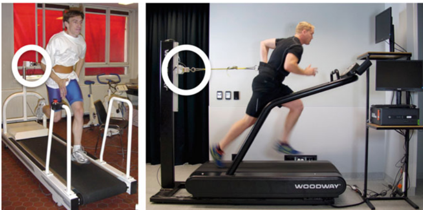
Fig. 10.1 Original (left) and modern (right) non-motorized treadmills. The pulling force is recorded via a load cell (white circles) and the running velocity is recorded via optical encoders installed in the rolling belt system
