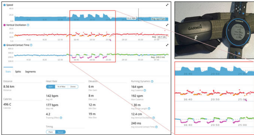
Fig. 8.11 Some sport watches such as the Garmin Forerunner 620™ include an accelerometer (Garmin HRM-Run™) carried at the chest (right). Contact time and other mechanical variables are then monitored for all steps of a run (left, example for a standard jog), allowing detailed follow-up of running mechanics, and calculation of the spring-mass variables using the simple method presented here. In this typical running session, five bouts of 1' run at maximal aerobic speed ( 20 \text{ km h}^{-1} ) and the associated changes in contact time and vertical oscillation of the center of mass appear in the red squares
