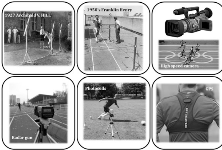
Fig. 11.1 Main devices used in the past and at the moment to analyse sprint kinematics out of labs
