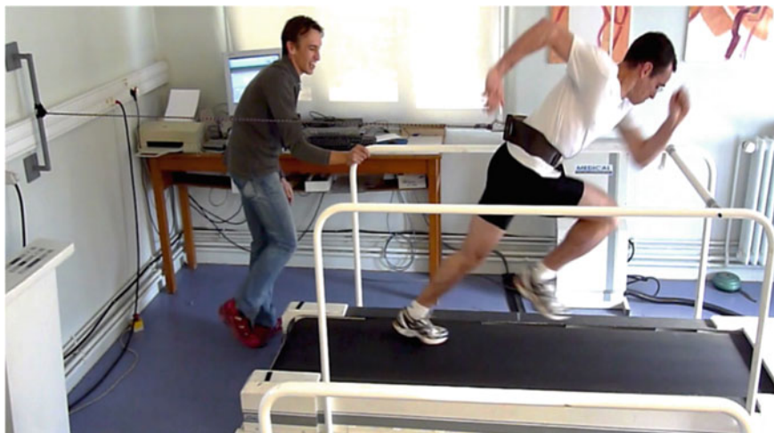
Fig. 10.4 Sprint instrumented motorized treadmill allowing direct and immediate changes in belt velocity following subject's actions during sprint acceleration, from null to maximal running velocity
