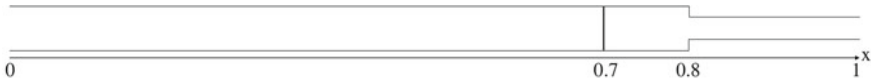
Fig. 2 Experimental setup: 1D pipe with a sudden contraction and position of the initial membrane
