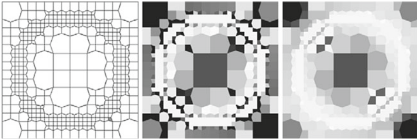
Fig. 3 Example 1 Left the consistent quadtree grid with the inspected element. For u_2(X) = \frac{1}{3}(x^3 + y^3) we compare (\nabla u)_p and (\nabla u)_p^A with the values of the gradient evaluated analytically in (x_p, y_p) . The values are scaled with darker values representing larger differences. Middle ||(\nabla u)_p^A| - |\nabla u_{exact}|| . Right ||\nabla u| - |\nabla u_{exact}||
