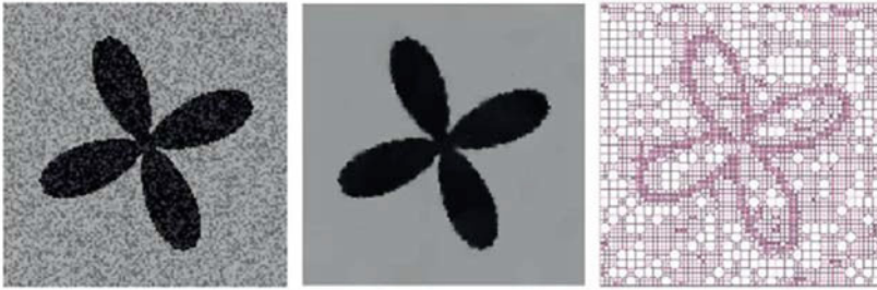
Fig. 4 Numerical experiment The artificial noisy image, the filtered image and the fixed adaptive grid
