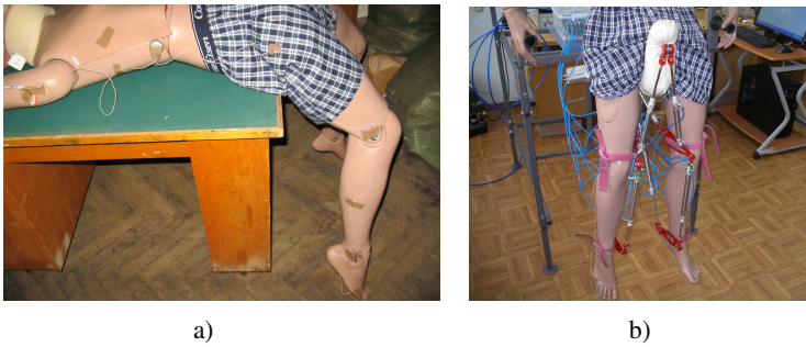
Fig. 5. Dummy with the markers as part of a model of the bio-mechatronic simulator. a) markers fixed on the dummy; b) the dummy as part of a model of the bio-mechatronic simulator.
