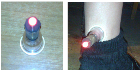
Fig. 2. Structure of the luminous marker (left: overall view, right: attachment to the human leg)
