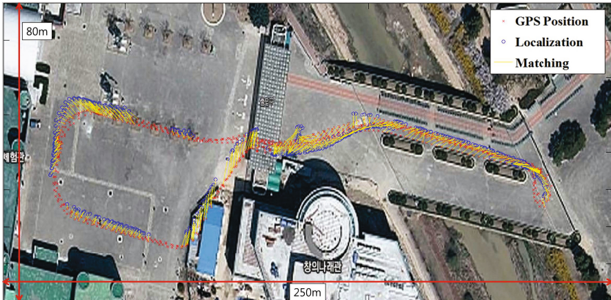
Fig. 5. The red crosses and blue circles indicate GPS position and the result of localization for full path. The yellow lines show matched result between them.
