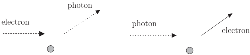
Fig. 2.18 Radiative recombination (left) and photoemission (right)
