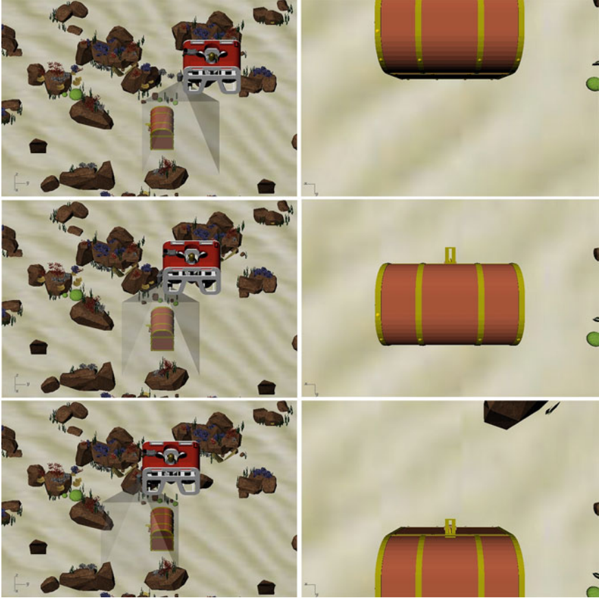
Fig. 1.2 Sequence corresponding to a straight trajectory of an AUV depicting the parallax problems. It shows the side and camera views of the robot's trajectory. One side of the chest disappears from the frame while the other arises due to the parallax effect
