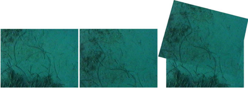
Fig. 2.3 Geometric registration of two different views of the same underwater scene by means of a planar transformation
