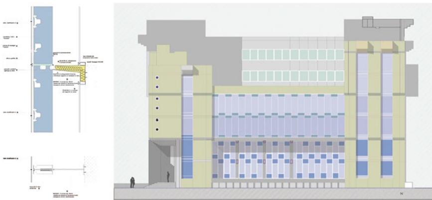
Fig. 11.7 Recovery project: vertical and horizontal section of double skin façade (on the left); overall view of the West elevation (on the right)
