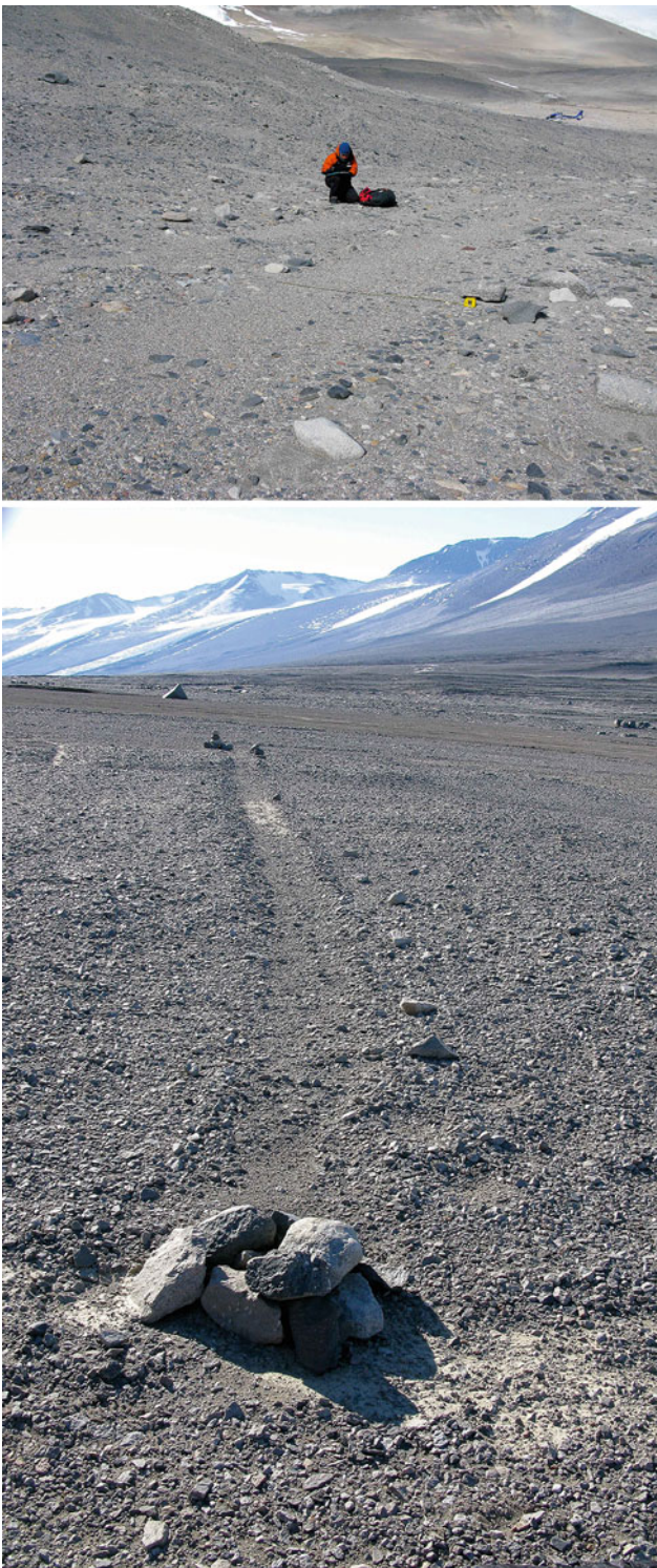
Fig. 15.5 An experimental treading trial on a fan near Lake Vanda in the Wright Valley illustrates the longevity of a walking track formed on gravelly sand fan materials. Top Site immediately after 200 walking passes in 1993. Bottom Same site revisited 17 years later in 2011. The pale coloured material visible on the track in photo b is fine sediment deposited by a recent fan-building event (Photos Megan Balks)
