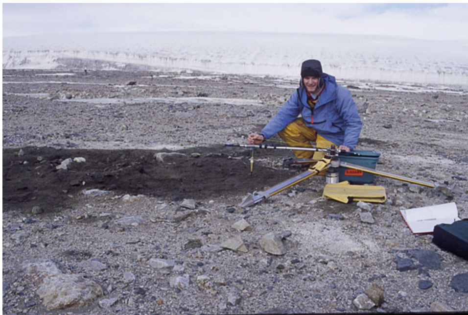
Fig. 15.9 Measurement of albedo on a surface darkened as a result of an oil spill about 40 years prior to the photo being taken ( Photo Taken January 2001 by Megan Balks )
