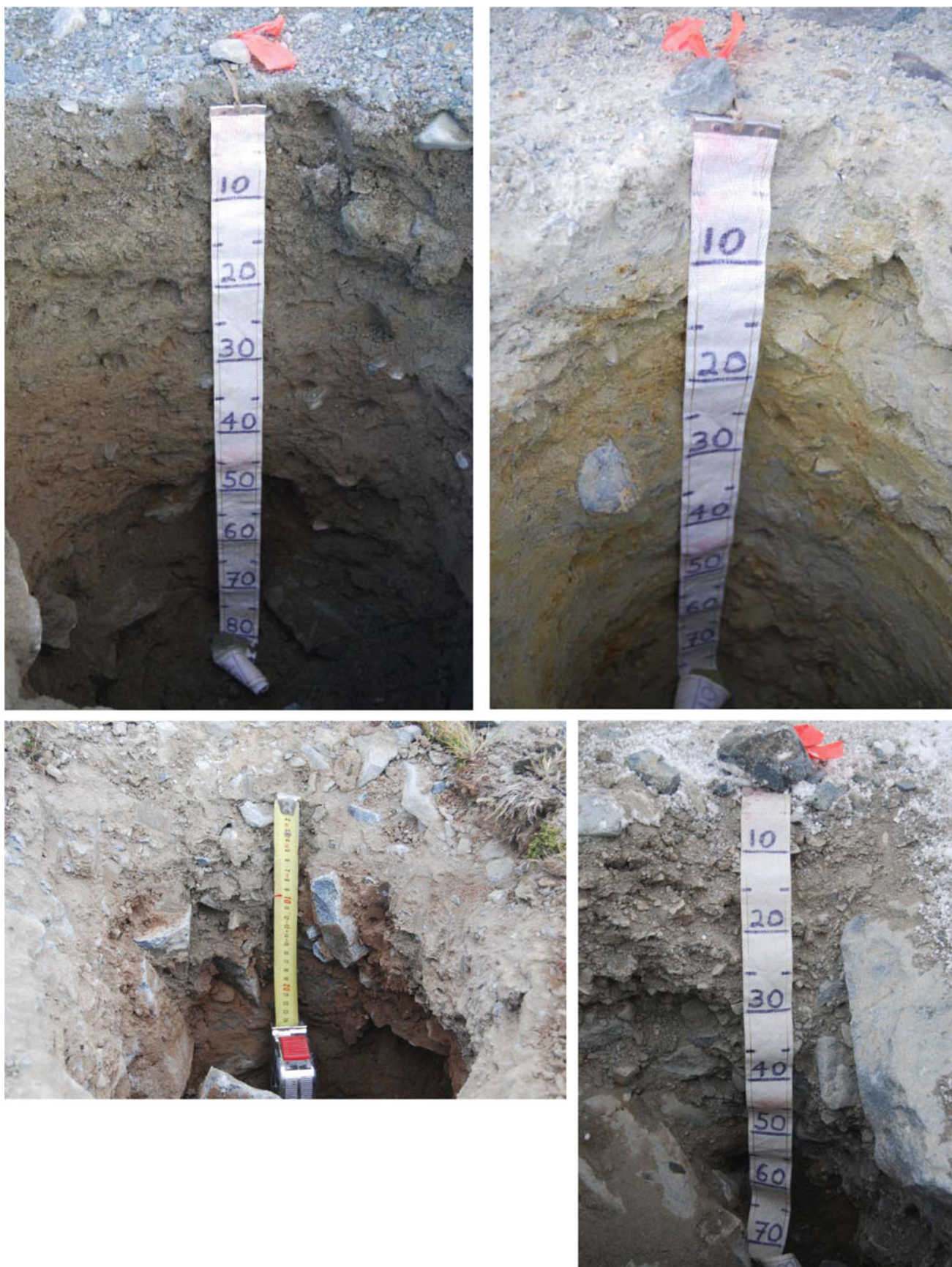
Fig. 12.7 Soils of Amsler Island, Palmer Archipelago, including Typic Gelorthents (A03, upper left ; A08, lower right ), a Typic Gelaquepts (A04, upper right ), and a Lithic Humigelepts (A05, lower left )
