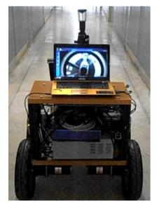
Fig. 1. An omnidirectional camera mounted on the mobile robot
