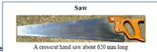
A crosscut hand saw about 620 mm long
