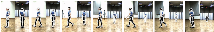
Fig. 5. Articulated 3D human body tracking in sequence P1S. Shown are results in frames #0, 20, 40, 60, 80, 100, 120. The left sub-images are seen from view 1, whereas the right ones are seen from view 2.
