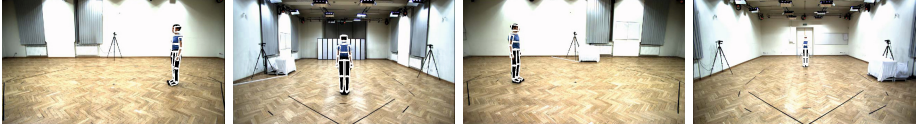
Fig. 3. Layout of the laboratory with four cameras. The images illustrate the initial model configuration, overlaid on the image in first frame and seen in view 1, 2, 3, 4.
