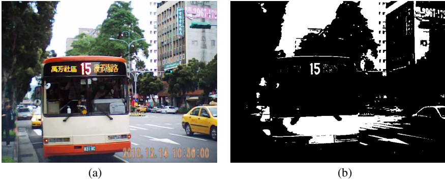
Fig. 1. Example of the bus route number detection. (a) The image of frame #26. (b) The image of thresholding result.
