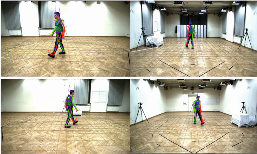
Fig. 4. An example of trial from dataset 4GAIT-MIS. Simultaneous visualization of data from mocap and four video streams.
