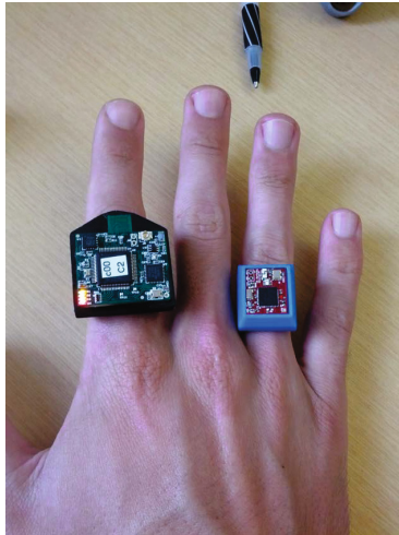
Fig. 4. Side by side comparison of two GINA boards
