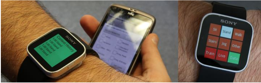
Fig. 3. Left: mobile phone running the novel framework and the SmartWatch showing prediction state (color) and behavioral history. Right: the view for labeling activities and controlling the framework state.
