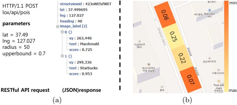
Fig. 16. (a) Request and response from REST API and (b) the heatmap showing the amount of changes
