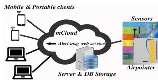
Fig. 1. Architecture of the Air Quality Monitoring System
