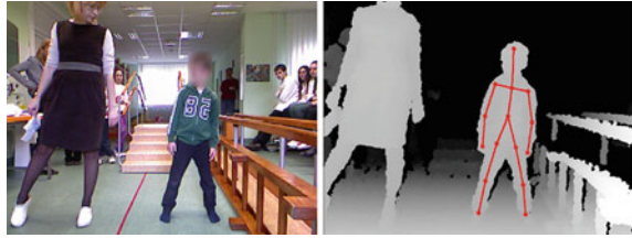
Fig. 2 Therapy session recording: left therapy setting; right recorded depth map with annotated tracked joints
