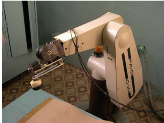
Fig. 7 Robot with position/force control for massage developed in Moscow State Industrial University
