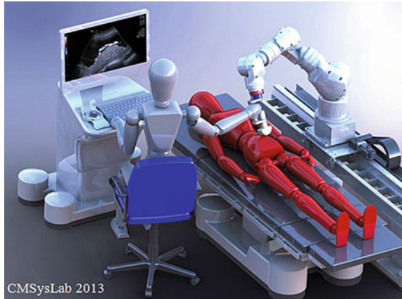
Fig. 11 Virtual model of a robot-assisted 3D medical sonography system, which is under development in the CMSysLab: active flexible humanoid arm—robot Yaskawa SIA 10F carries the ultrasound probe and, through various modes of interactive operation, enables a wide range of behaviours in a cooperative sonographer–robot–patient system
