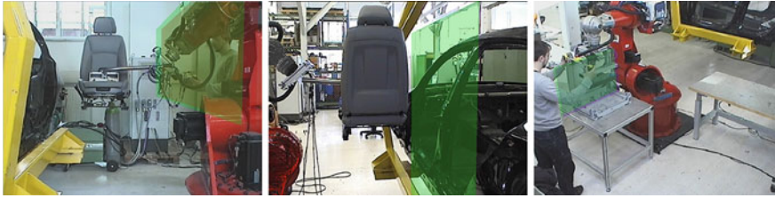
Fig. 5 Virtual barriers visualized using augmented reality, acting as safety boundaries during transport or as assistance stops during assembly
