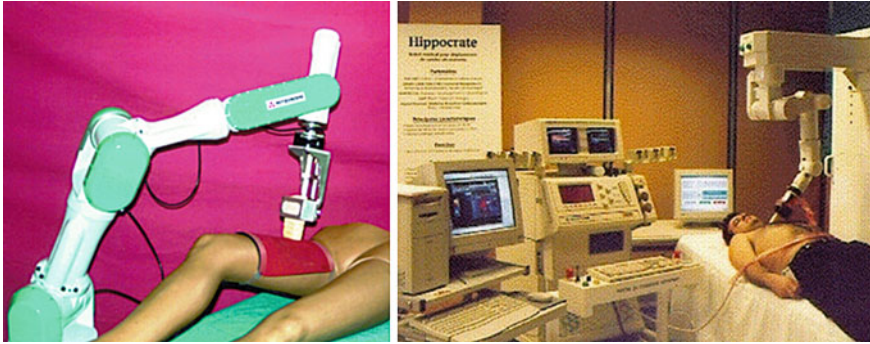
Fig. 1 The Hippocrate project: test table with force controlled Mitsubishi PA-10, 7 d.o.f. robot ( left ), and dedicated 6. d.o.f. Hippocrate robot in the environment for 3D US rendering of major blood vessels geometry ( right )
