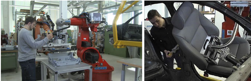
Fig. 7 The Fit4Work assistance system used in industrial use cases for assembly of dishwasher counter-weights and a car seat
