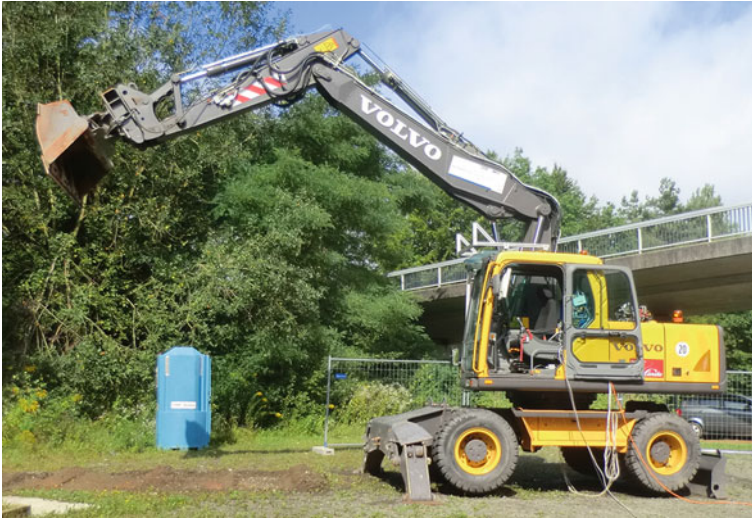
Fig. 1 The autonomous bucket excavator THOR ( Terraforming Heavy Outdoor Robot )
