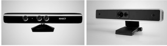
Fig. 1 Sample 3D sensors for indoor applications: left Microsoft Kinect for Windows (Microsoft Corporation 2013), right Softkinetic DepthSense 311 (SoftKinetic 2013)
