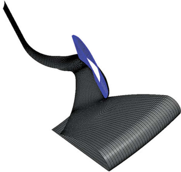
Fig. 3 Mesh generated for a single blade passage
